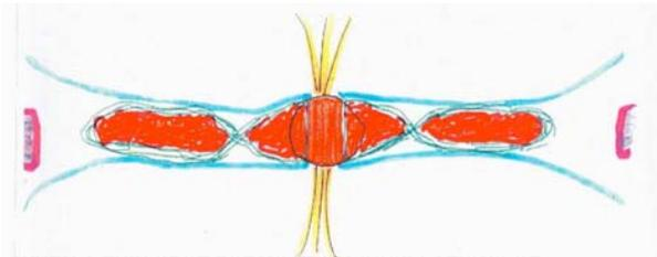
WHEN A THIN SPOT FORMS FROM OSCILLATIONS OR WHATEVER, THE MAGNETIC FIELD LINES CAN RECONNECT.
