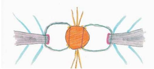
**MAGNETIC FIELD IS STRETCHED OUTWARD WITH THE DISK SINCE IT IS PINNED TO THE DISK. AS THE COUPLING WEAKENS THE FIELD LINES WRAP.**
